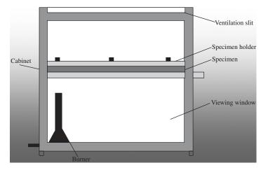
Figure 1. Schematic of FMVSS 302 fire test.
